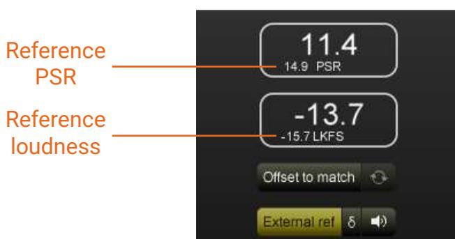
Place MasterCheck as you usually would to monitor your mix and click the 'External ref.' button. If you are using more than one NUGEN Audio SEND plug-in in your mix, you may need to open the settings panel and select the correct source from the drop down menu.
