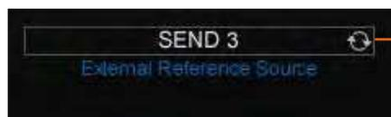
Click to sync MasterCheck with SEND plug-in to remove delays caused by plug-in Latencies FX chain.
